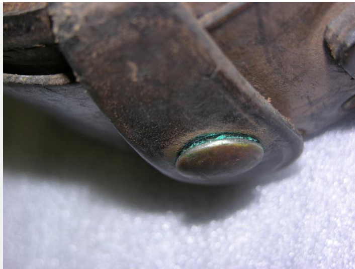
Green corrosion is often seen when copper alloys touch leather due to oils in the leather. This reaction is exacerbated by leather dressings.
