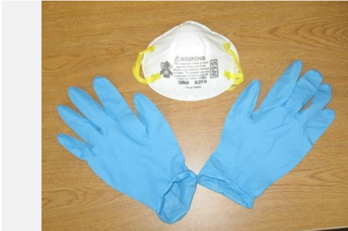
Nitrile gloves and a dust mask is the right personal protective equipment (PPE)
