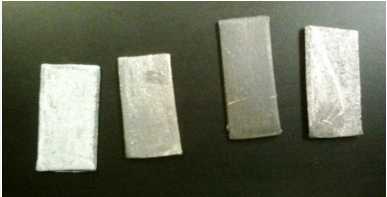
From left to right: lead exposed to plywood has powdery white corrosion, lead exposed to Brilliantize had little change, lead exposed to CRL had a significantly darkened surface, and our lead coupon from the clean jar for comparison.
