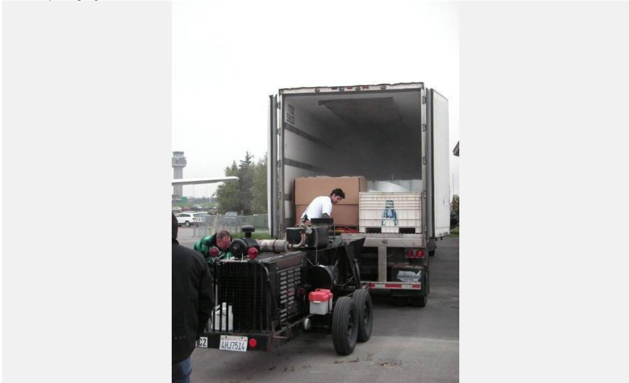
Half a semi-trailer with ice blocks, which are chopped into “snow” by the diesel-powered black machine in the foreground.
